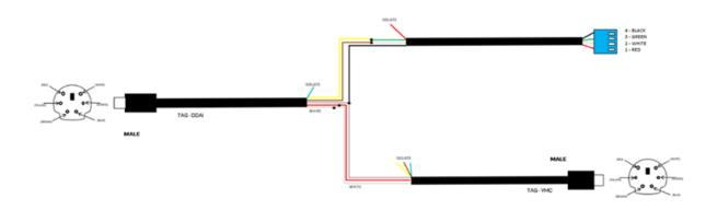
• The 6PDM-SERIAL-Y cable then connects to the serial port of the DVR and one of the camera channels (specified in install schematic).
